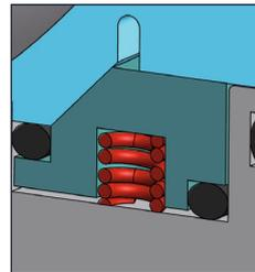
**2. Spring loaded sealing system**
