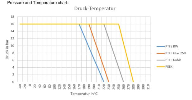
By ignoring these limit values, improper use of the compact- valve is the consequence and could lead to failure of the valve function.
